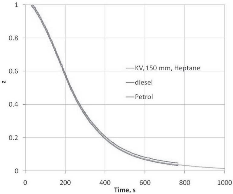
Figure 9 Drained fraction vs time, for KV AFFF foam with heptane, petrol and diesel liquid-foam interfaces.
