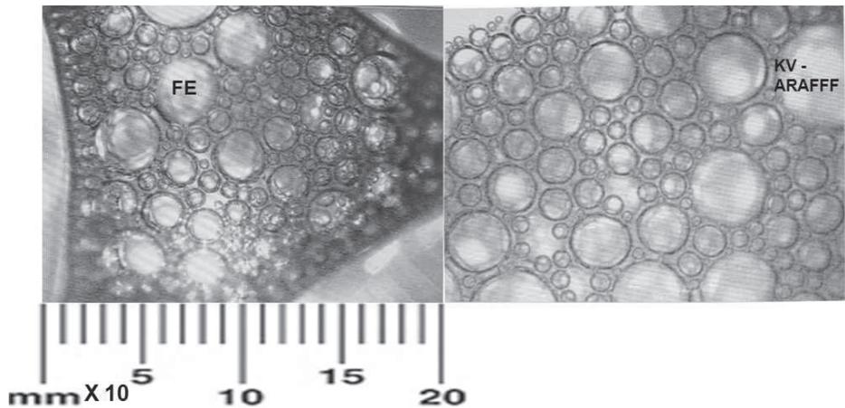
Figure 5 Foam bubbles under a microscope - FE and KV AR-AFFF
