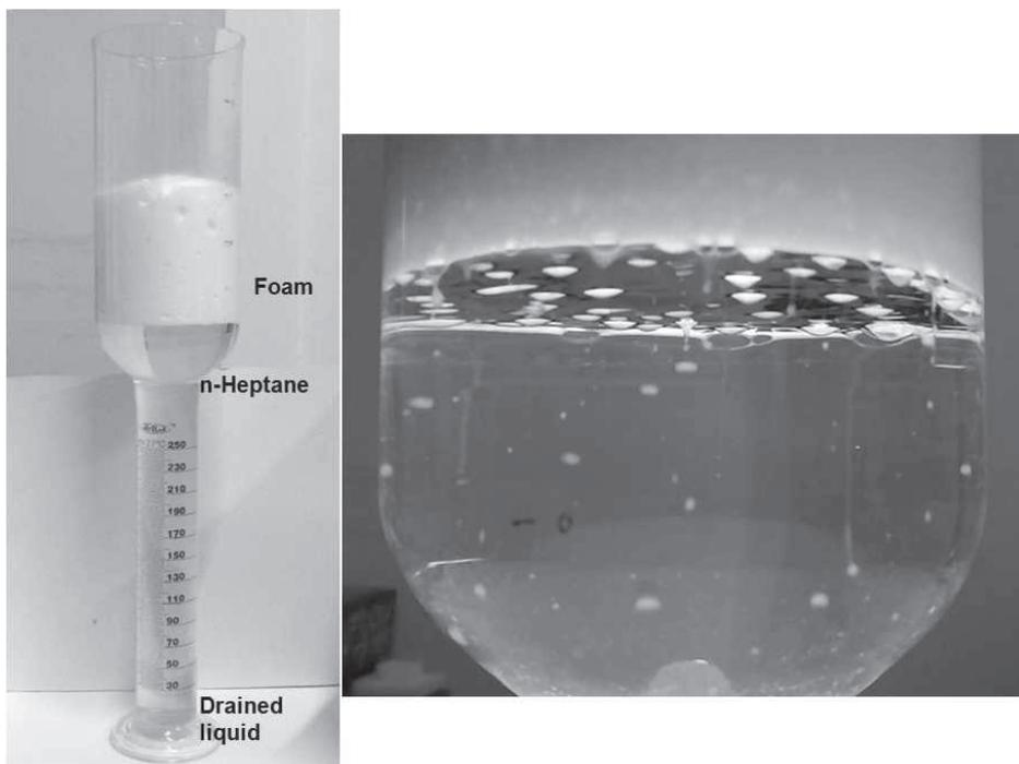
*Figure 1 The foam drainage apparatus (left) and the drainage process (right)*
