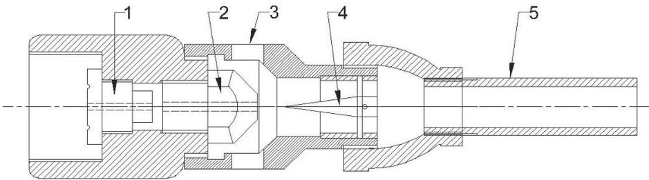
*Figure 3* Foam nozzle used to generate the foam
